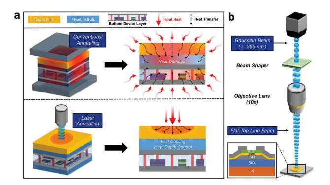
Annealing method for M3D integration processes a) Schematic illustration comparing the heat distribution in multi-layer devices between laser annealing and conventional annealing. b) Schematic of the laser system with device structure. Credit: *Advanced Science* (2024). DOI: 10.1002/advs.202401250
