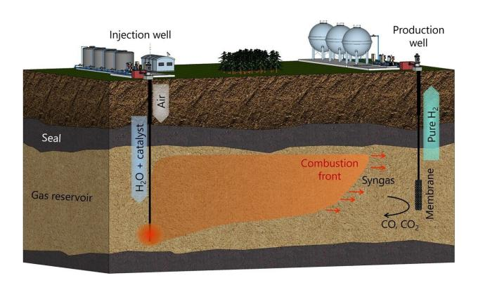
The process of hydrogen production from gas fields. Credit: Mukhina et al. / Fuel, 2024
