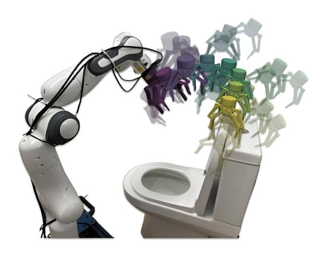
A high-level overview of the Render and Diffuse process in the context of a putting the toilet seat down task. Rendered robot grippers are updated iteratively using a learnt denoising process until they represent actions needed to complete the task. Different colors represent different robot actions in the future. Credit: Vosylius et al.
