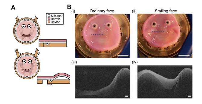
The new anchoring method allows flexible skin tissue to conform to any shape it's attached to. In this case, a relatively flat robotic face is made to smile and the skin deforms without constraining the robot, returning to its original shape afterwards. Credit: 2024 Takeuchi et al. CC-BY-ND
