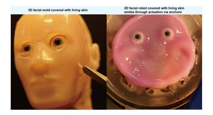
Other methods to bind skin tissue to solid structures come with limitations. This new method can work on complex, curved, and even moving surfaces. Credit: 2024 Takeuchi et al. CC-BY-ND
