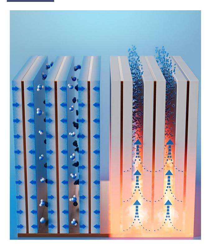
A simple, compact system first collects moisture from the air (left) and then releases the trapped liquid (right) when heated, which results in potable water. Credit: Xiangyu Li
