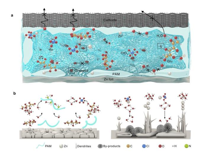
a. Schematic illustration of the design and construction of electrolyte structure;b. Schematic illustration of Zn plating behavior in Glu/ZC/PAM (left) and pure ZC (right). Credit: Li Zhaoqian
