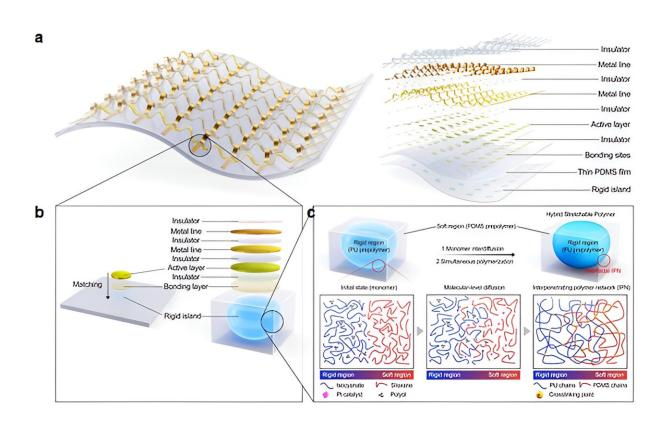
Interpenetrating polymer (IPN)-based stretchable substrate and integrated electronics system. Credit: DGIST (Daegu Gyeongbuk Institute of Science and Technology)
