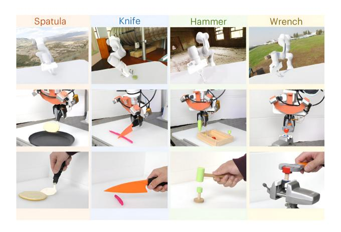
Three different data domains — simulation (top), robot tele-operation (middle) and human demos (bottom) — allow a robot to learn to use different tools.
