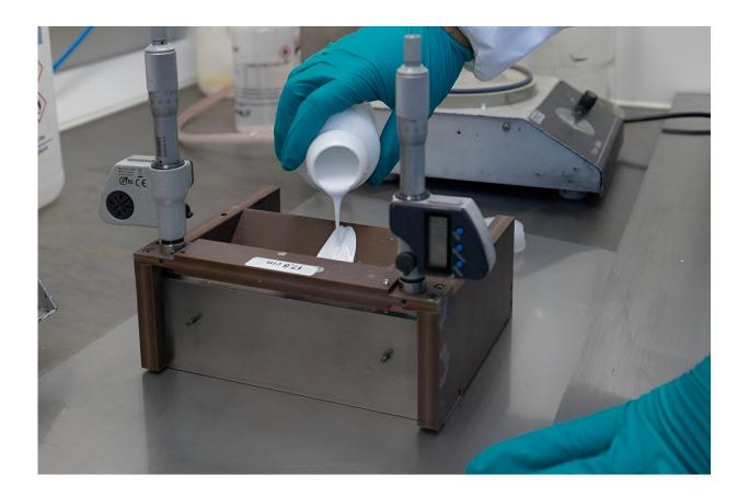
The powder is mixed with a binder and a solvent and the liquid solution is poured onto a roller that rolls out the material in a thin layer. The quality of the solution is assessed to make a solid electrolyte with fewer defects. Credit: Frida Gregersen
