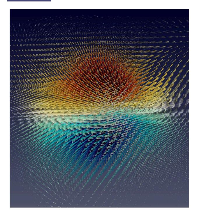
Skyrmion-like large hole polaron in the halide double perovskite Cs2AgBiBr6. The arrows show the atomic displacements, and the hole is at the center of this vortex. The displacement field has defined topological character, with integer topological charge and vorticity. Credit: J. Lafuente-Bartolome.
