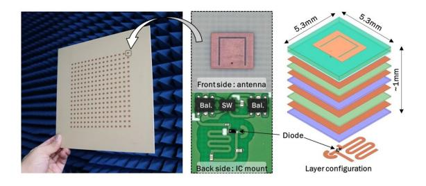
The proposed transceiver design enables high power conversion efficiency and conversion gain, enhancing 5G network coverage even in areas with link blockage. Credit: 2024 IEEE MTT-S International Microwave Symposium
