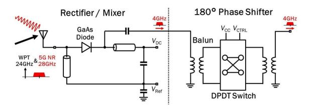
The board includes gallium arsenide diodes, balun ICs, DPDT switch ICs, and digital ICs. This circuit generates DC from 24GHz WPT signal and downconverts 28GHz RF signal to 4GHz IF signal simultaneously. Credit: 2024 IEEE MTT-S International Microwave Symposium
