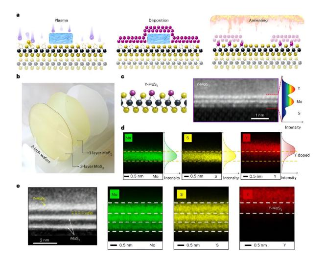
Fabrication and characterization of two-dimensional metallization. Credit: *Nature Electronics* (2024). DOI: 10.1038/s41928-024-01176-2
