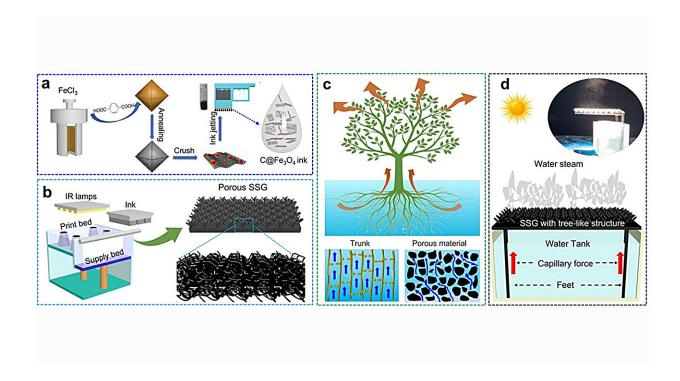
The fabrication and application of MJF-printed SSGs. (a) Synthesis process of the C@Fe3O4 ink for MJF printing. (b) Illustration of the MJF testbed setup and the structure of printed SSGs. (c) Schematic illustration of transpiration in plants and water transport in trunk and porous materials. (d) The illustrated evaporation process of water on the surface of MJF-printed SSG under solar irradiation. Credit: Yanbei Hou et al.
