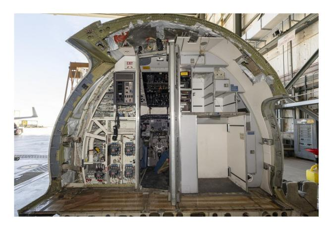
The cockpit of an old MD-90 aircraft arrived at NASA's Armstrong Flight Research Center in Edwards, California, in March 2024. Parts will be used to build a simulator for NASA's X-66, the demonstration aircraft for the Sustainable Flight Demonstrator project. Credit: NASA/Steve Freeman
