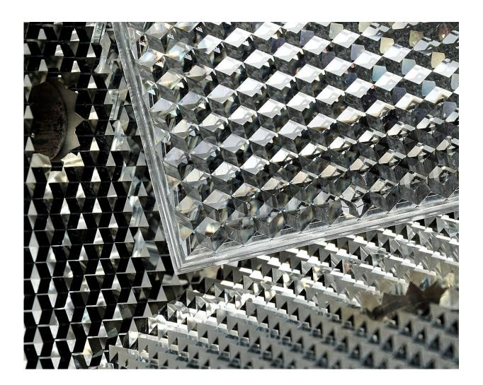
UltraPLAS enables perfect reproduction of mirror-finish surfaces. Releasecoated tool (l.) with injection-molded element. Credit: Fraunhofer IFAM/Wolfgang Hielscher
