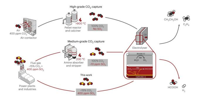
Processing of CO<sub>2</sub> gas. The capture and electrolysis of CO<sub>2</sub> from air or flue gas
