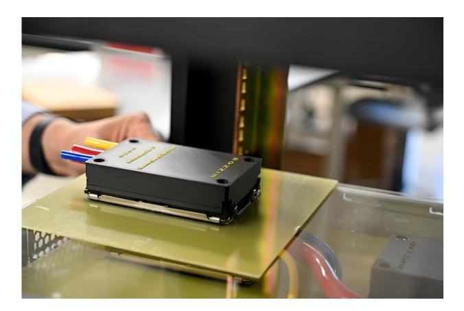
The cooling system dissipates heat from server chips through phase change, such as boiling a liquid into vapor in a thin, porous layer. Credit: University of Missouri
