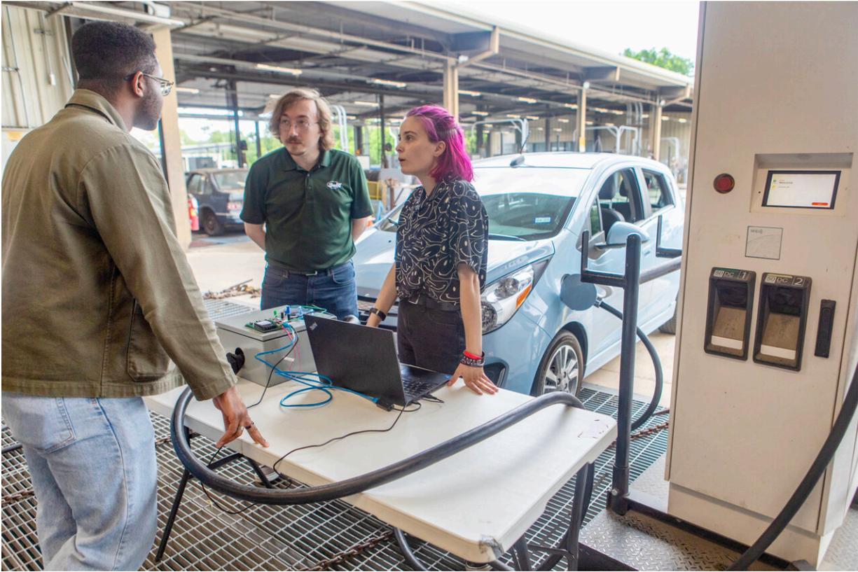
SwRI research engineers, from left, FJ Olugbodi, Mark Johnson and Katherine Kozan demonstrate an adversary-in-the-middle device they developed to test the cyber resiliency of ISO 15118-compliant vehicle-to-grid charging systems. With the device, SwRI identified cybersecurity vulnerabilities with electric vehicles using direct current fast-charging systems. Credit: Southwest Research Institute
