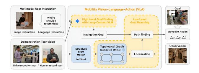
Mobility VLA architecture. The multimodal user instruction and a demonstration tour video of the environment are used by a long-context VLM (high-level policy) to identify the goal frame in the video. The low-level policy then uses the goal frame and an offline generated topological map (from the tour video using structure-from-motion) to compute a robot action at every timestep. Credit: arXiv (2024). DOI: 10.48550/arxiv.2407.07775
