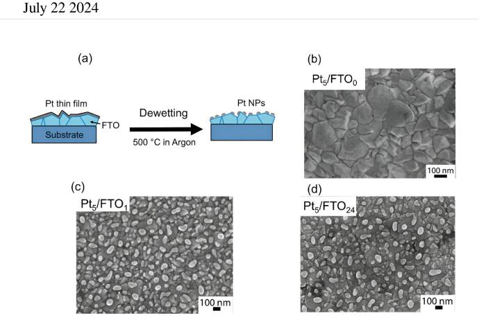
Schematic representation for dewetting of Pt thin films on FTO upon heat treatment at 500 °C in argon. SEM micrographs of b) as-deposited Pt thin film,  $Pt_5/FTO_0$ , c)  $Pt_5/FTO_1$  and (d)  $Pt_5/FTO_{24}$ . Credit: *Advanced Functional Materials* (2024). DOI: 10.1002/adfm.202403628
