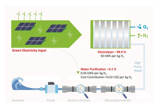
Comparison of the energy and overall costs of seawater purification and electrolysis. Credit: N. Hausmann/HZB in Joule
