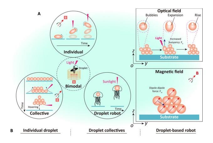
Schematic and experiment snapshots showing the individual and assembling behavior of bimodal droplets. Credit: *Science Advances* (2024). DOI: 10.1126/sciadv.adp1439
