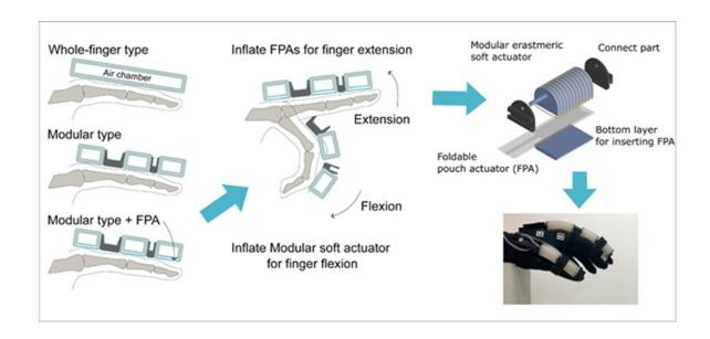
Chiba University researchers succeeded in overcoming limitations associated with finger straightening or extension without compromising existing functionality of finger bending or flexion through design improvements in soft rehabilitation gloves—they developed a novel foldable pouch actuator that seamlessly integrates with existing soft actuators used in the gloves. Credit: Professor Wenwei Yu / Chiba University, Japan
