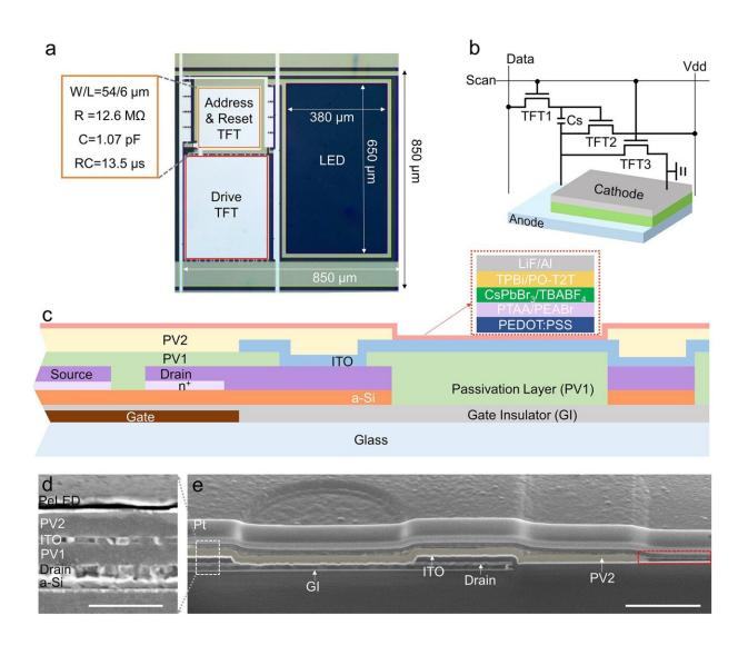
Structure of AM PeLED. a, Micrograph of one single pixel in the TFT backplane showing the layout of TFT and LED area. b, The schematic diagram
