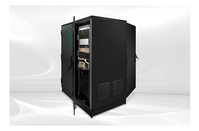
AQT has realized the first quantum computer compatible with standardized 19"-rack infrastructure. These systems can be readily installed at HPC or data centers. Operating at room temperature with a power consumption of less than 2 kW, this eco-friendly quantum computer offers the highest quantum volume within Europe. Credit: Dieter Kühl/AQT
