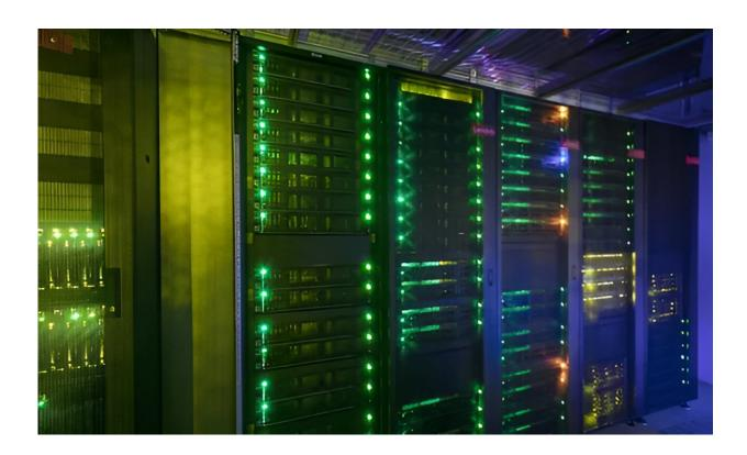
The HPC cluster LEO 5 at the University of Innsbruck offers up to 250 billion computing operations per second. User access, resource management and process flow follow international standards and are therefore compatible with other HPC facilities. Credit: University of Innsbruck
