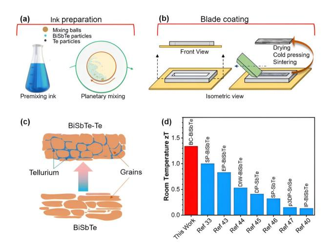
(a) Schematic representation of the thermoelectric ink formulation. (b) Blade coating for fabricating thick thermoelectric films. (c) Schematic of the Te-assisted liquid-phase sintering of BiSbTe. (d) Comparison of room-temperature zT between our blade-coated BiSbTe–Te sample and other p-type thermoelectric materials made with different ink-based processes. Credit: *Energy & Environmental Science* (2024). DOI: 10.1039/D4EE00866A
