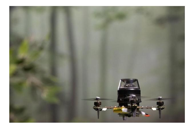
The proposed insect-inspired navigation strategy allowed a 56-gram "CrazyFlie" drone, equipped with an omnidirectional camera, to cover distances of up to 100 meters with only 0.65 kiloByte. Credit: Guido de Croon / TU DelftlMAV Lab
