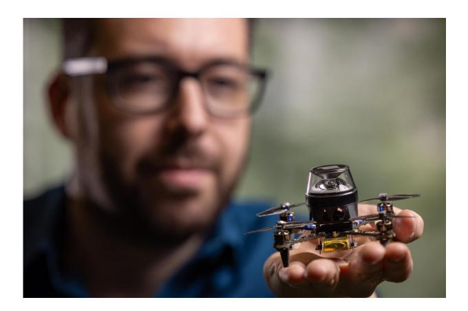
Tiny, 56-gram "CrazyFlie" drone that is able to navigate back to a starting location with an insect-inspired navigation strategy. Credit: Guido de Croon / TU Delftl MAV Lab
