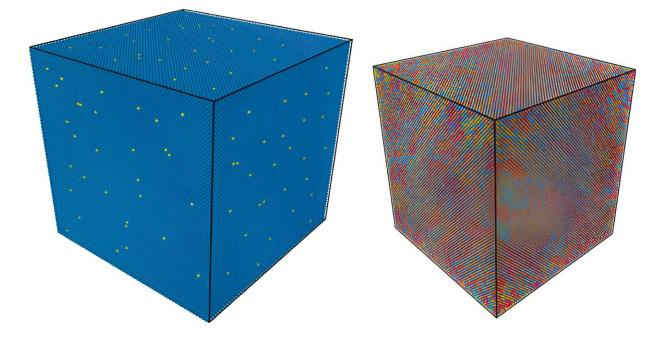
On the left, a traditional alloy with a main element in blue and a small amount of a different element in yellow. High-entropy alloys (as seen on the right) contain several elements in nearly equal amounts (three in this figure), creating many possibilities for chemical patterns. "It's like you're making a recipe with a lot more ingredients," says Yifan Cao, on of the authors of the paper, but it also adds significant chemical complexity. Credit: Massachusetts Institute of Technology
