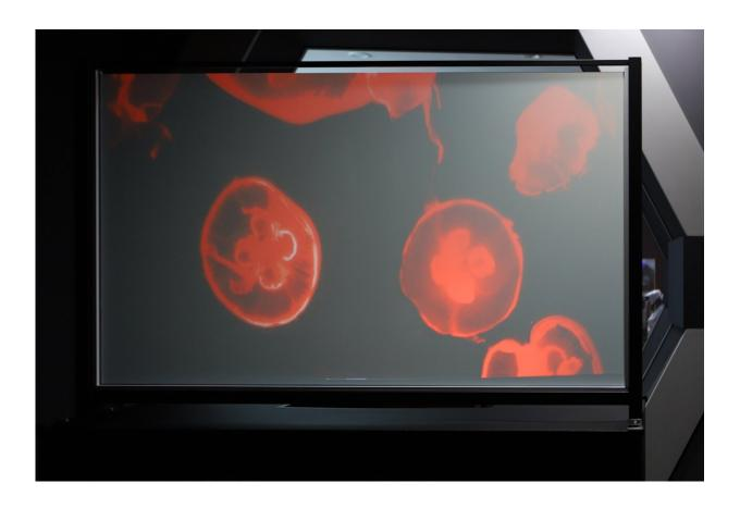
Image of the large-sized NTS, jointly developed by the KIMM and Meta2People, being demonstrated (semitransparent). Credit: Korea Institute of
