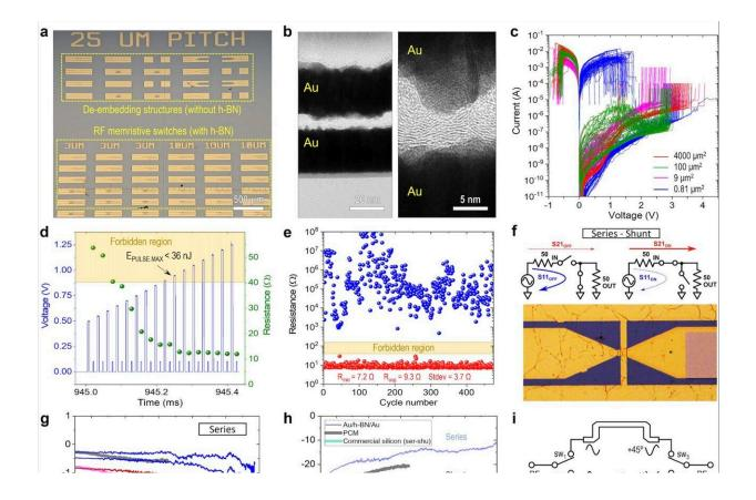
a, Optical microscope image of a meta/h-BN/metal array and RF de-embedding structures. b, Cross-sectional TEM images of a Au/CVD h-BN/Au device, showing layered structure. c, Characteristic I-V curves displaying at least 100 consecutive cycles for each device area. d, Conductance-enhancing protocol using 10  $\mu$ s voltage pulses. e, Variability resistance through 475 cycles of a single device switched following the protocol from d. f, Circuit schematic and optical
