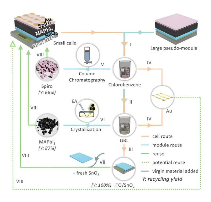
Schematic diagram of closed-loop recycling of perovskite solar devices. Credit:
