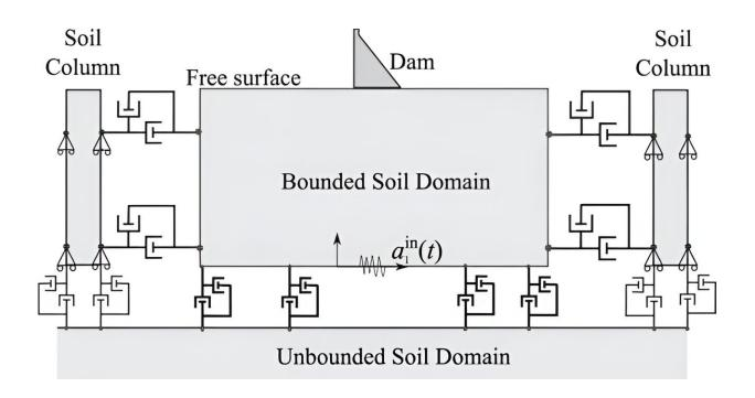
Finite element model for seismic analysis of concrete dam soil. Credit: *International Journal of Mechanical System Dynamics* (2024). DOI: 10.1002/msd2.12106
