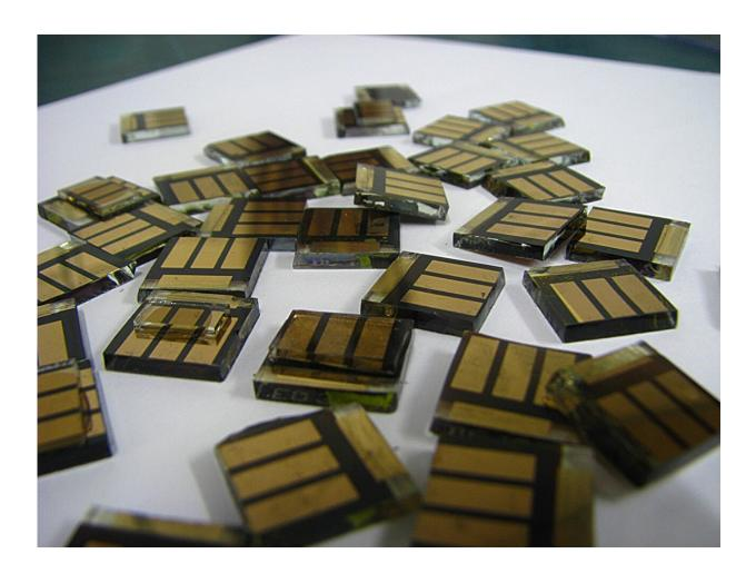
Using 4PTSC as a multifunctional additive greatly improves crystal growth in tinhalide perovskites, reducing the number of defects that typically hamper efficiency. Moreover, thanks to the chemical properties of this compound, oxidation and moisture infiltration are minimized, which boosts the durability of the material. Credit: University of Oxford Press Office. https://openverse.org/image/279011b5-abb4-47c9-9e28-e5b002d50b7a
