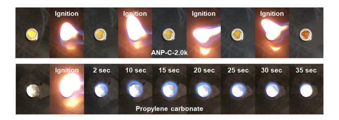
The flame tests depict that the new electrolyte membrane (above) is not ignited even with multiple applications of an open flame and resultingly simply turns into coal ash, in contrast with the highly flammable liquid organic solvent (below). Credit: The University of Hong Kong
