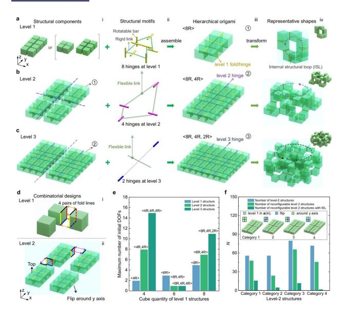
Design of hierarchical origami-based shape-morphing metastructures. Credit: *Nature Communications* (2024). DOI: 10.1038/s41467-024-50497-5
