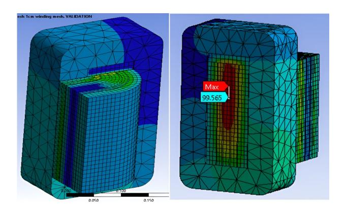
Predicting hot spots inside a transformer. Internals of transformers can get as hot as boiling water (100°C). Credit: Vaibhav Bahadur, UT Austin
