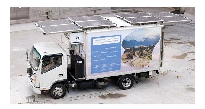
Installed on the roof, the extensible solar photovoltaic panels can be extended to increase the freezer truck's power output, enhancing its energy efficiency. Credit: 2024 Research and Innovation Office, The Hong Kong Polytechnic University. All Rights Reserved.
