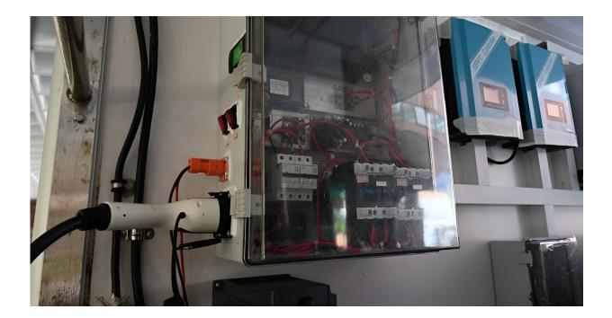
The truck is equipped with an energy storage device that captures and stores the electric energy generated, providing additional energy for the vehicle's freezer system. It also has an onboard lithium-ion battery that can be connected to standard electric vehicle charging facilities for recharging. Credit: 2024 Research and Innovation Office, The Hong Kong Polytechnic University. All Rights Reserved.
