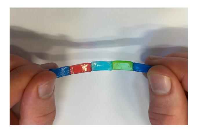
Researchers have developed soft, stretchable 'jelly batteries' that could be used for wearable devices or soft robotics, or even implanted in the brain to deliver drugs or treat conditions such as epilepsy. Credit: University of Cambridge
