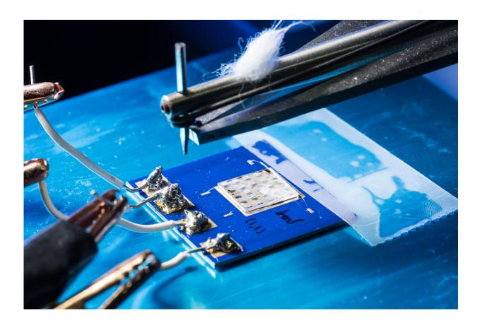
Rochester researchers demonstrated their super-high resolution thermometry techniques on an electrical heater structure that the team designed to produce sharp temperature gradients. Credit: University of Rochester / J. Adam Fenster
