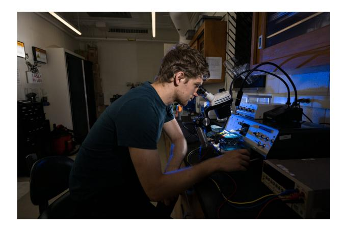
Materials science Ph.D. student Benjamin Harrington uses a wire bonder to add electrical connections to an electrical heater structure. The structure was designed as a test subject for a new heat mapping technique that leverages Nobel Prize in Chemistry–winning optical super-resolution fluorescence microscopy techniques. Credit: University of Rochester / J. Adam Fenster
