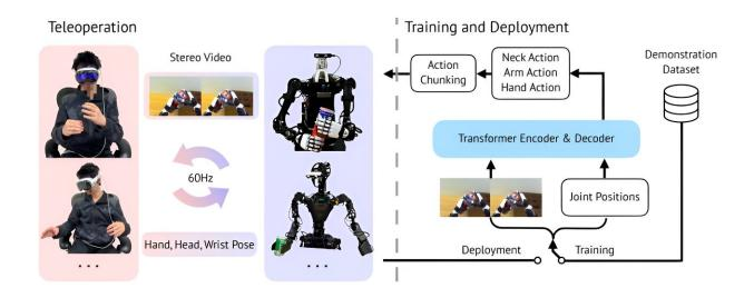
Teleoperated data collection and learning setup. Left: our teleoperation system. Right: we train an imitation policy for each task with action chunking transformer. The transformer encoder captures the relationship of image and proprioception tokens and the transformer decoder outputs action sequences of a certain chunk size. Credit: *arXiv* (2024). DOI: 10.48550/arxiv.2407.01512
