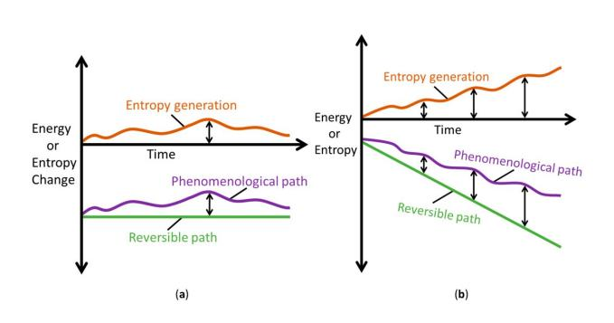
Illustrations of the Phenomenological Entropy Generation theorem, showing reversible (green) and phenomenological (purple) paths; the vertical difference between the paths (see black arrows) defines entropy generation or energy dissipation (orange). (a) Rates and (b) Accumulations. Credit: *Entropy* (2024). DOI: 10.3390/e26030237
