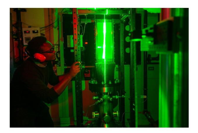
UC aerospace engineer Vincent Onoja peers through a glass window in a jet engine illuminated with a laser. He developed an experimental method to study airflows in jet engines that uses a high-speed camera to record the aerosol particles as they travel through the engine. Credit: Andrew Higley/UC Marketing + Brand
