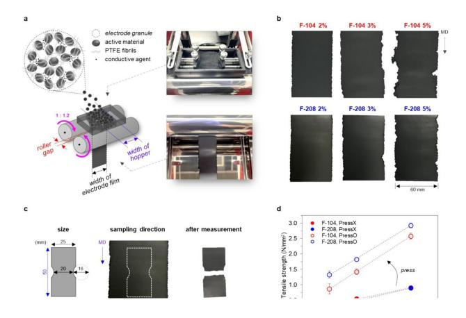
Film formation—roll mill—electrode film. (a) Schematic of the manufacture of electrode film from electrode granules using a roll mill. (b) Photographs of the electrode film by type and amount of PTFE after roll milling. Credit: *Chemical Engineering Journal* (2024). DOI: 10.1016/j.cej.2024.151957
