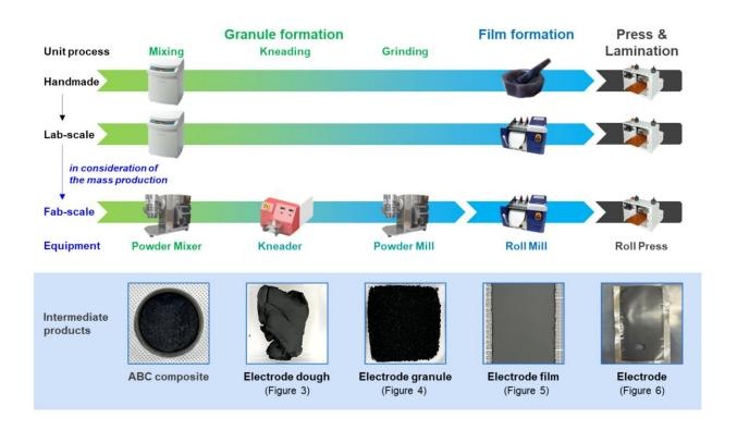
Overview of dry electrode manufacturing process: unit processes, equipment, and intermediate products used in this study. Credit: *Chemical Engineering Journal* (2024). DOI: 10.1016/j.cej.2024.151957
