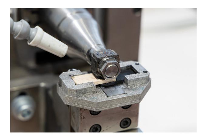
In Ultrasonic Joining, wood and the base component are joined by frictional heat. Credit: Wolf - TU Graz
