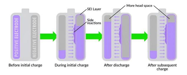
Factory-charging a new lithium-ion battery with high currents significantly depletes its lithium supply but prolongs the battery's life, according to research at the SLAC-Stanford Battery Center. The lost lithium is generally usually used to form a protective layer called SEI on the negative electrode. However, under fast charging conditions, lithium ions are also consumed during side reactions at the negative electrode. This creates additional headspace in both electrodes and
