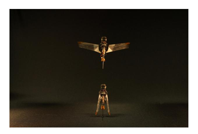
The flapping microrobot takes flight with passive deploying-retracting wings. Credit: Hoang-Vu Phan
