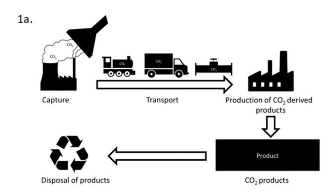
1a) Process of carbon capture and utilization. Credit: *Sustainable Production and Consumption* (2024). DOI: 10.1016/j.spc.2024.08.003
