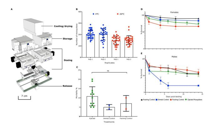
Mosquito dosing and quality from the automated release mechanism. Credit: Ya-Hsun Lin et al, *Science Robotics* (2024). DOI: 10.1126/scirobotics.adk7913
