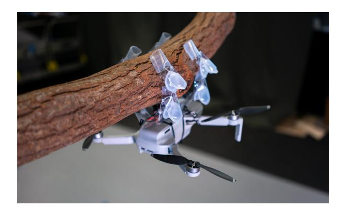
FiBa soft gripper mounted on a DJI quadcopter, demonstrating its enhanced capability to perch securely on a branch. Credit: SUTD
