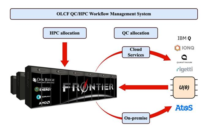
Schematic of the QC/HPC integration at OLCF. This is a high-level view of the ideal state of the framework presented in Section 8. The framework will integrate simulators, cloud-based quantum devices, and on-premises quantum hardware in a seamless way. Credit: *Future Generation Computer Systems* (2024). DOI: 10.1016/j.future.2024.06.058
